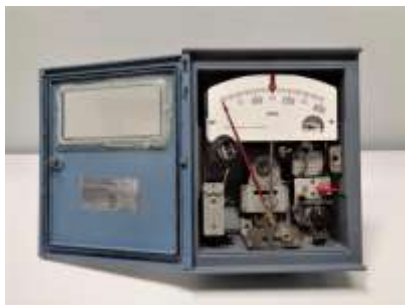
Foxboro pneumatic controller First pneumatic controller 1930
