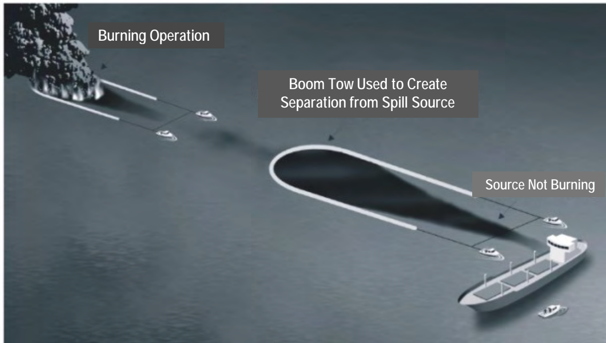
Figure 23 - Use of Towed Boom to Burn and to Separate Source from Fire
