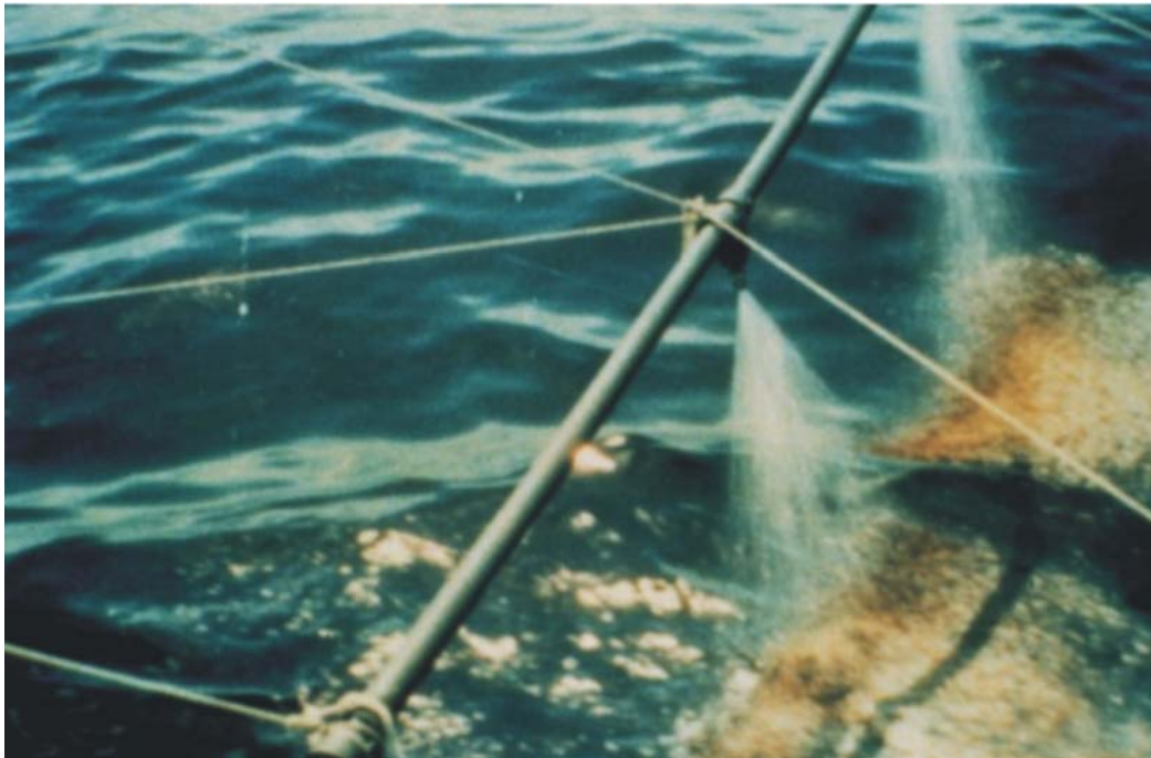
Figure 1: A spray system from a boat in operation (Note the underlapping spray pattern)
