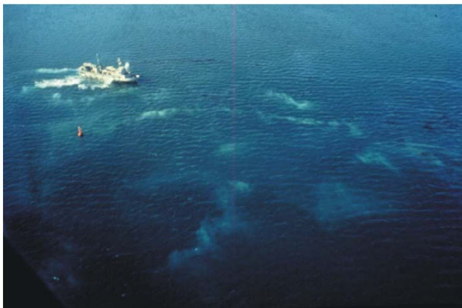
Figure 6: View of a dispersant application where dispersant-only plumes are seen Part of this is caused by ineffectiveness on the heavy oil coming from the ship
