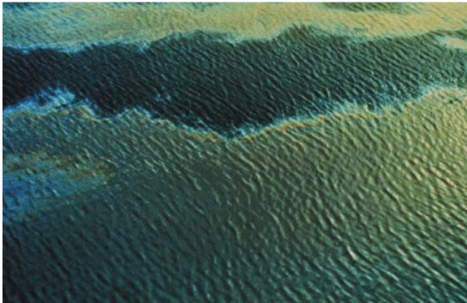
Figure 6: View of a dispersant application where dispersant-only plumes are seen Part of this is caused by ineffectiveness on the heavy oil coming from the ship
