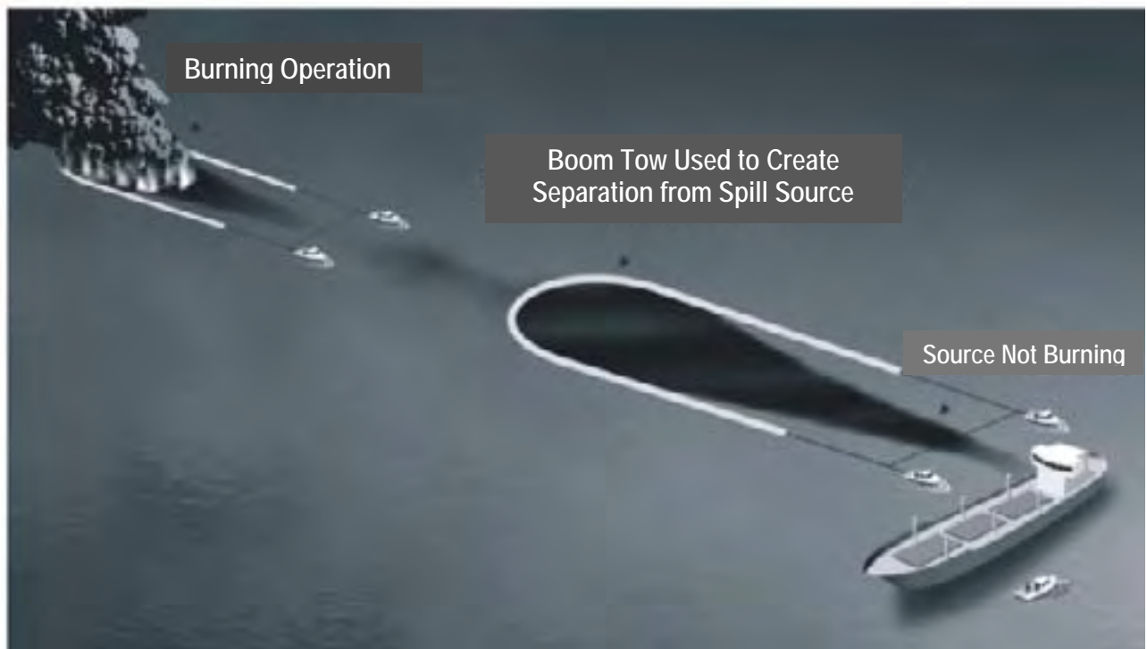
Figure C3: Use of Towed Boom to Burn and to Separate Source from Fire
