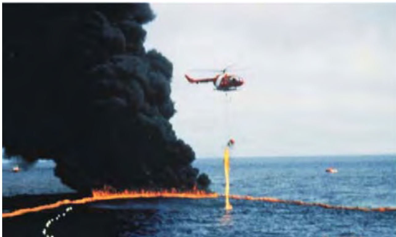
Figure 10: A Helitorch in operation. In general, an ignition device must meet two basic criteria in order to be effective. It must apply sufficient heat to produce enough oil vapors to ignite the oil and then keep it burning and it must be safe to use. The most sophisticated commercial devices used today for igniting oil slicks are the helitorch igniters. These are helicopter-slung devices that dispense packets or globules of burning, gelled fuel and produce an 800 °C flame that lasts up to 6 minutes.
