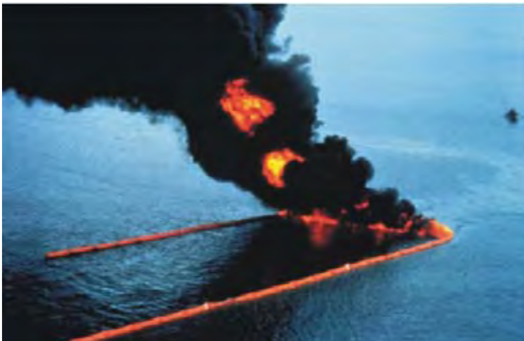
Figure 8: A test burn at sea. Note that the boom was incorrectly towed downwind and there is some leakage behind the boom
