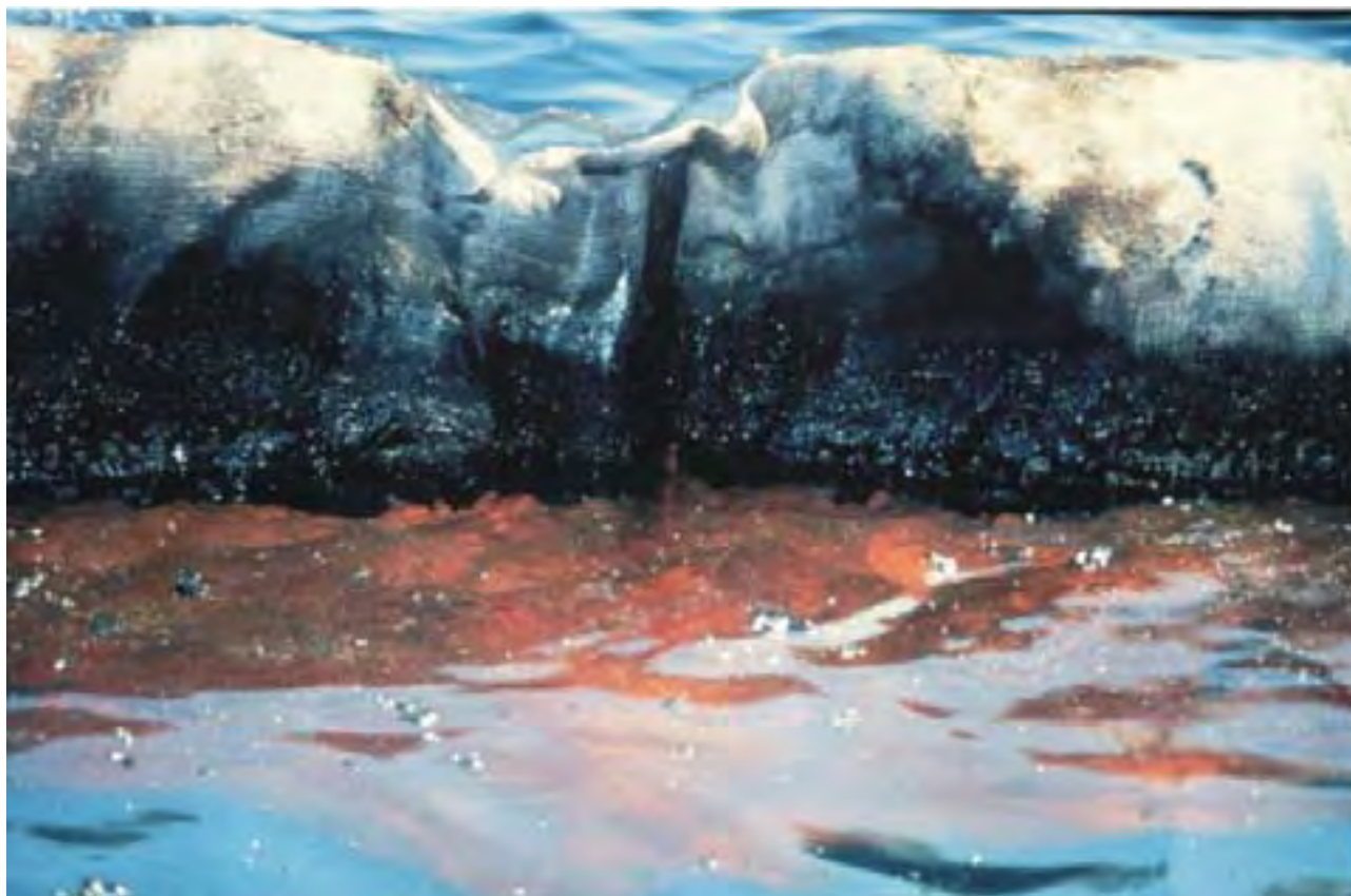
Figure 11: This is the residue remaining from a 50-ton burn at sea. The oil residue is from a light to medium crude oil. The residue is relatively heavy which is shown by the small amount of water on top of the residue. The fire-resistant boom is an older technology, with a mesh covered with a fire-resistant material.
