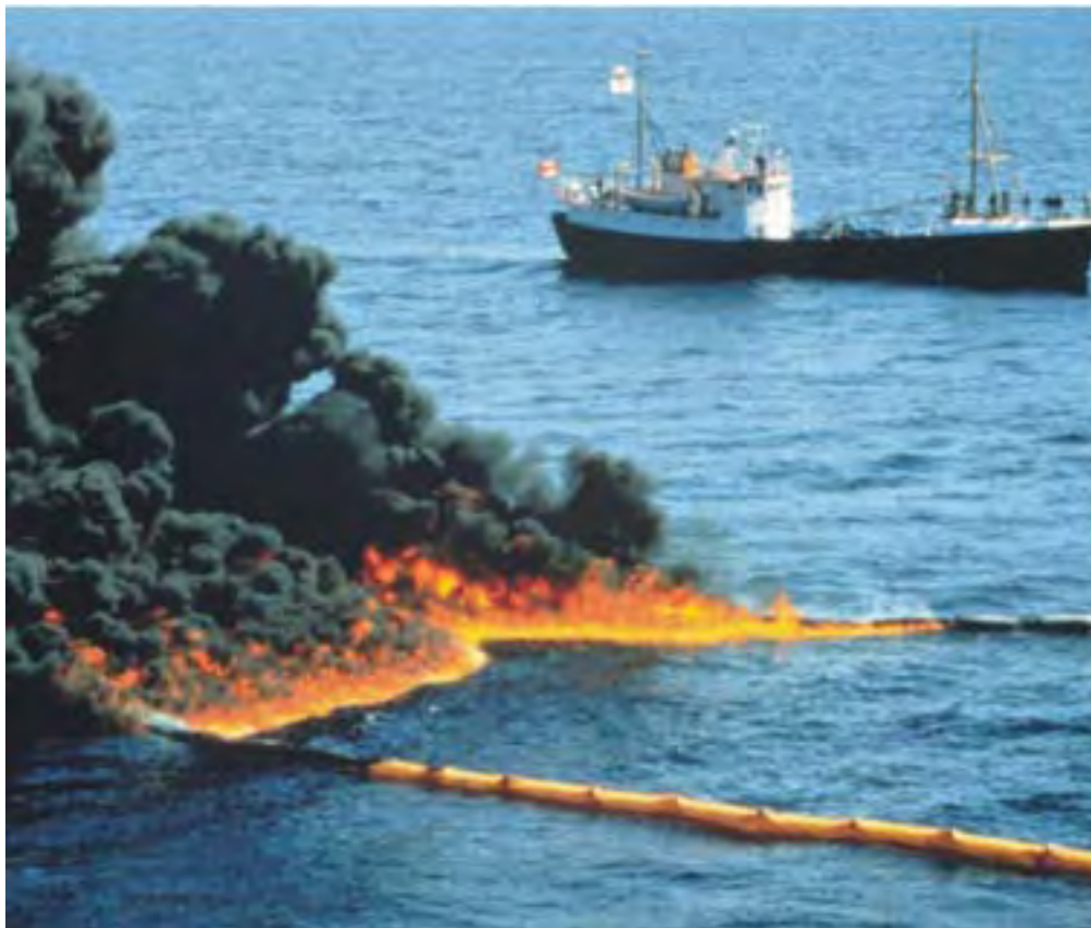
Figure 7: A test burn at sea using a fire-resistant boom for containment. At the time this picture was taken, only oil at the rear of the slick is burning, as the forepart is too thin.
